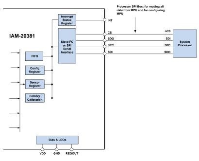
Figure 7. IAM-20381 Solution Using SPI Interface
