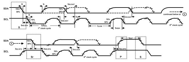
Figure 1. I<sup>2</sup>C Bus Timing Diagram
