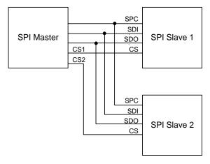
Figure 11. Typical SPI Master/Slave Configuration
