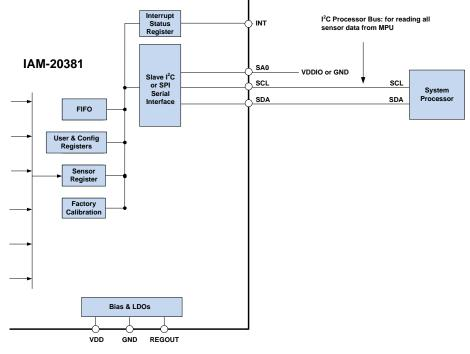
Figure 6. IAM-20381 Solution Using I<sup>2</sup>C Interface
