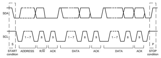
Figure 10. Complete I<sup>2</sup>C Data Transfer
