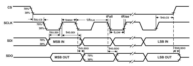
Figure 2. SPI Bus Timing Diagram
