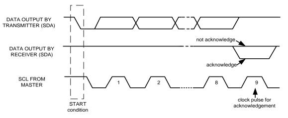
Figure 9. Acknowledge on the I<sup>2</sup>C Bus
