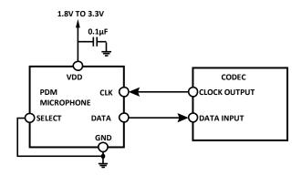
Figure 10. Mono PDM Microphone (Right Channel) Connection to Codec
