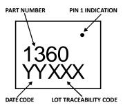
Figure 16. Package Marking Specification (Top View)
