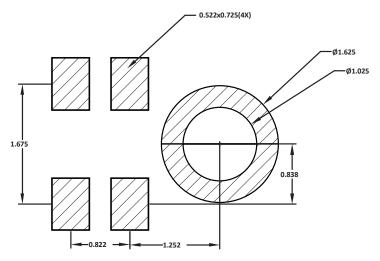
Figure 13. Recommended PCB Land Pattern Layout
