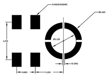
Figure 14. Suggested Solder Paste Stencil Pattern Layout
