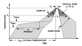
**Figure 2. Recommended Soldering Profile Limits**
