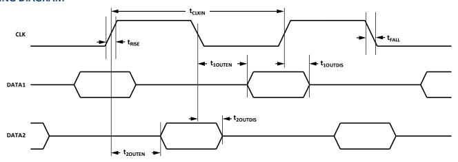
Figure 1. Pulse Density Modulated Output Timing
