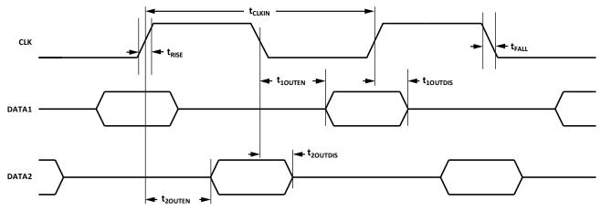
Figure 1. Pulse Density Modulated Output Timing
