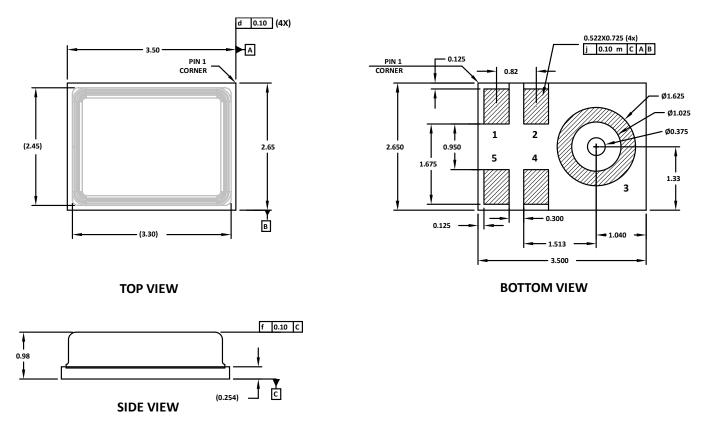
Figure 18. 5-Terminal Chip Array Small Outline No Lead Cavity [LGA\_CAV] 3.5 mm × 2.65 mm × 0.98 mm Body Dimensions shown in millimeters Dimension tolerance is ±0.15 mm unless otherwise specified
