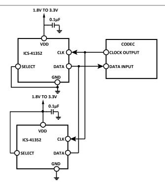
Figure 14. Stereo PDM Microphone Connection to Codec
