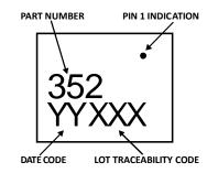
Figure 19. Package Marking Specification (Top View)
