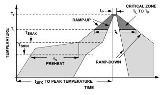
Figure 2. Recommended Soldering Profile Limits
