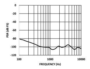
Figure 6. Power Supply Rejection (PSR) vs. Frequency
