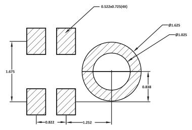
Figure 16. Recommended PCB Land Pattern Layout
