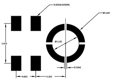
Figure 17. Suggested Solder Paste Stencil Pattern Layout
