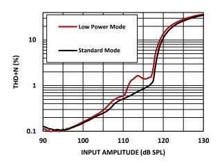
Figure 5. THD + N vs. Input Level
