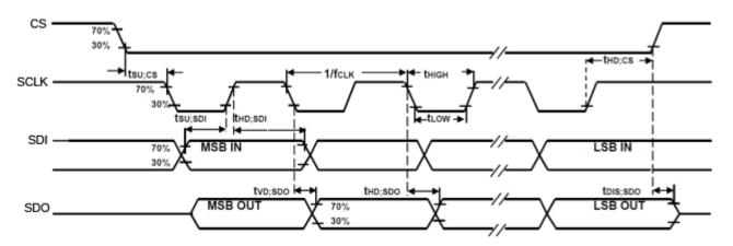
**SPI Bus Timing Diagram**
