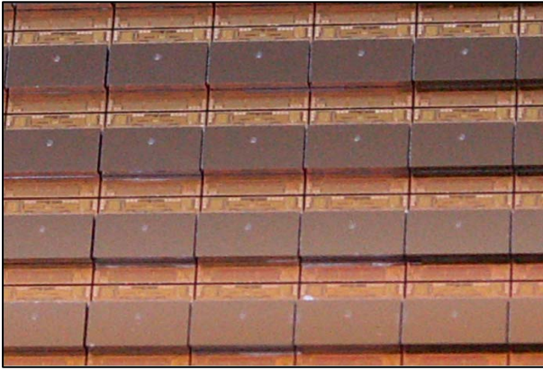
Figure 11. InvenSense's dual-axis gyro after dicing and pad
