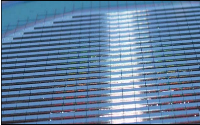
Figure 7. InvenSense's complete MEMS gyro wafer with batch processed wafer-scale integration
