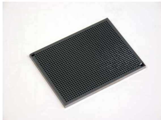
Figure 8: Tree layer of MEMS' integrated at wafer level to make 1200 fiber positioner
