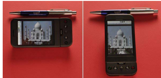
Figure 3. Gyroscopes enable portrait-landscape mode switch when device is placed on the table.
