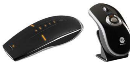
Figure 4. The Logitech® MX™ Air Mouse and the Air Mouse Elite™ from Gyration both feature inertial sensors for air mouse functionality and optical sensors for standard 2D mouse functionality. 7,8
