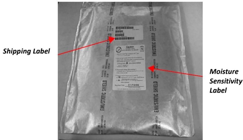
Figure 15. Moisture Sealed Reel
